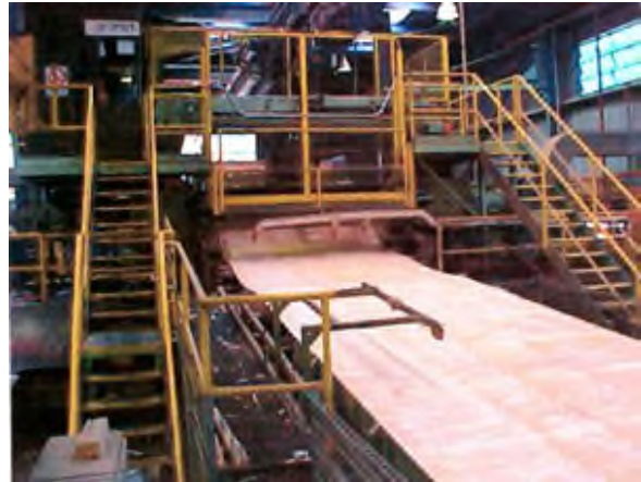
Veneer ribbon exiting lathe after peeling
