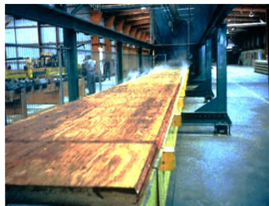
LVL production line
