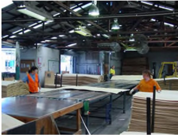
After drying, the veneer is sorted into grades ready for lay-up
