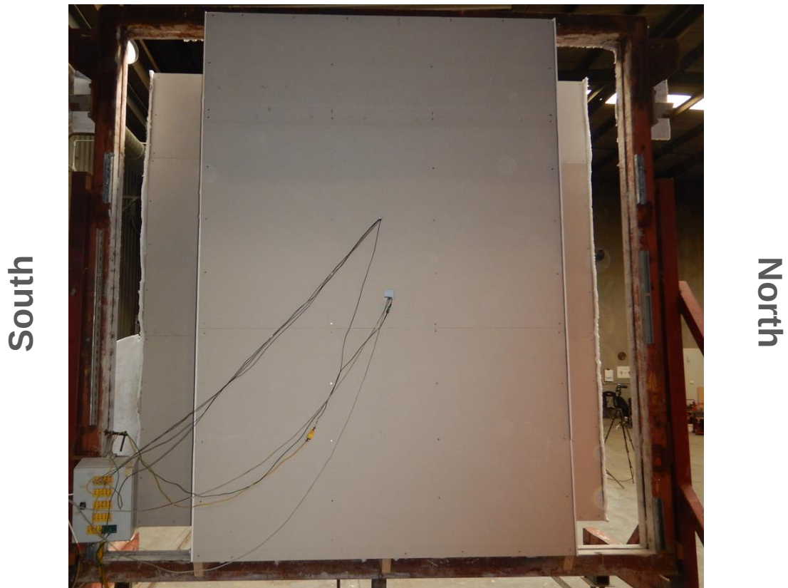
Figure 6 Unexposed face of the specimen at the end of the test
