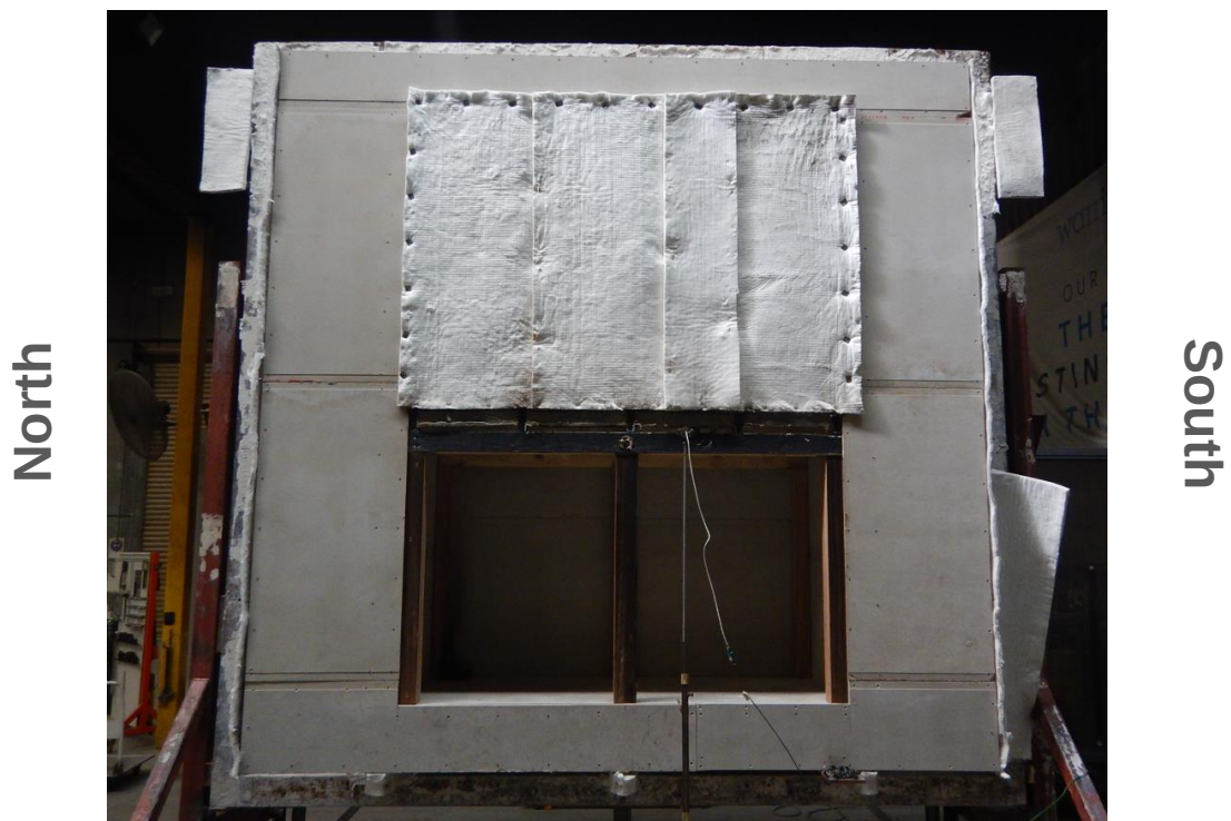
Figure 7 Exposed face of the specimen at the end of the test
