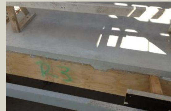
Timber-concrete composite floor
