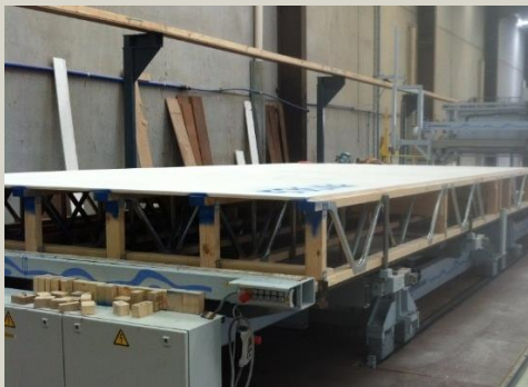
Floor cassette line
