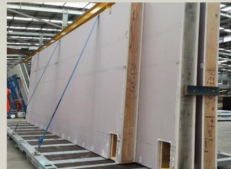
Fully enclosed staggered stud walls
