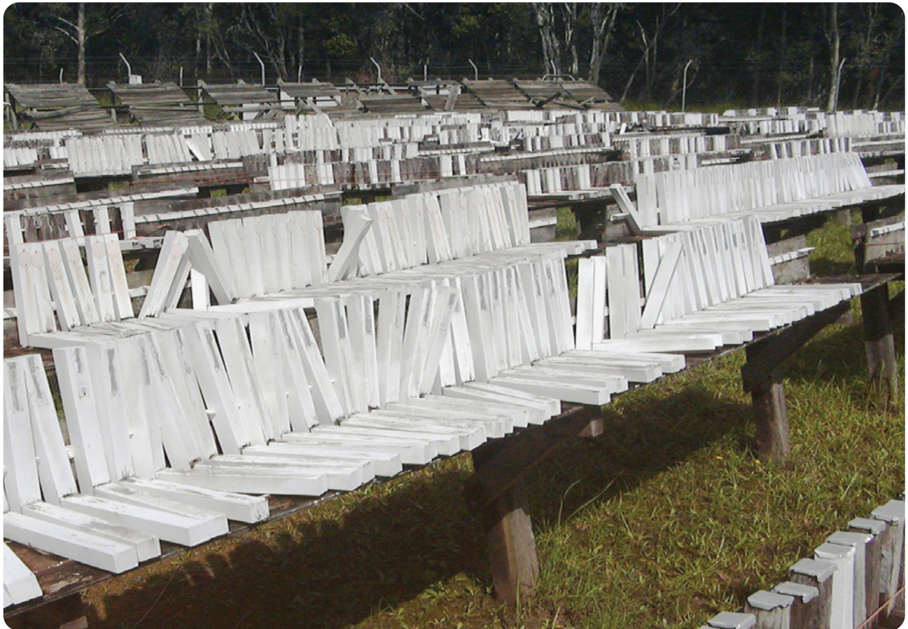
Above-ground durability test site in South-East Queensland.
