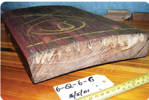
Section of stair tread showing poor maintenance has led to premature decay.
