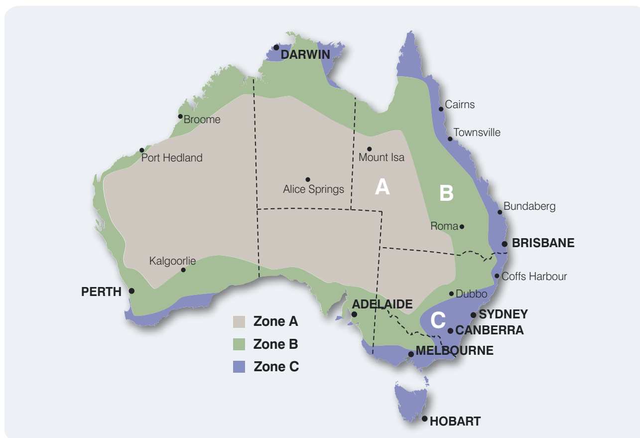
Figure 8.2: Hazard zone for embedded corrosion.
