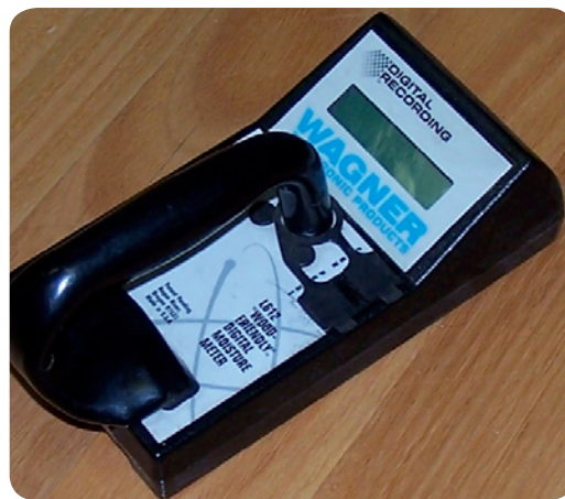
Left: Figure B2: Capacitance moisture meter - Measures average moisture – Need to set species density.
