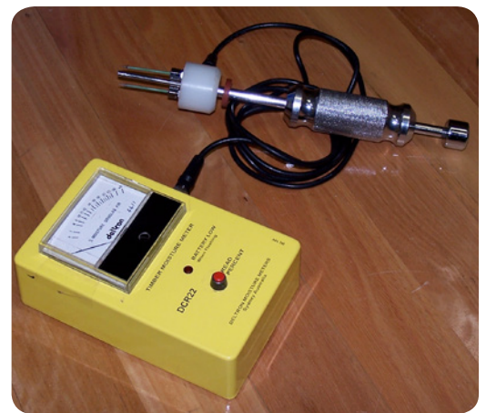
Left: Figure B2: Capacitance moisture meter - Measures average moisture – Need to set species density.
