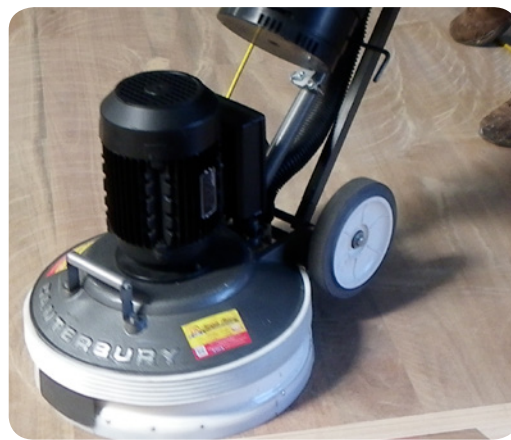
Figure 8.7: Hard plating with the correct attachment.
