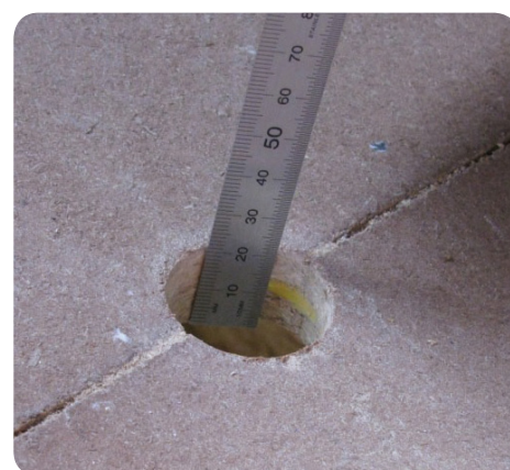
Measuring the thickness of particleboard flooring at a hole saw sample location.
