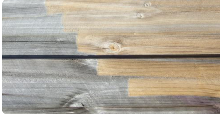
Figure 9: Weathered, grey surface adjacent to unweathered surface.
