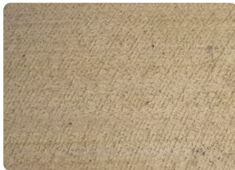
Rough sawn (circular saw).
