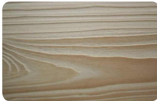
Figure 2.5: Wire-brushed surface of CLT. Photograph: PlanetArk
