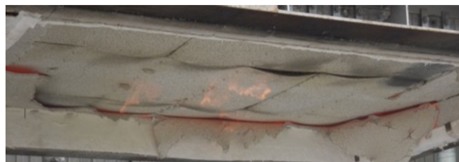
Fire-exposed face after removal from the furnace
