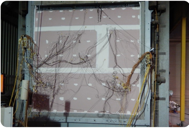
Figure 119: Non-fire side of specimen 229 min after commencement of test showing no visible degradation (heating terminated at 227 min).
