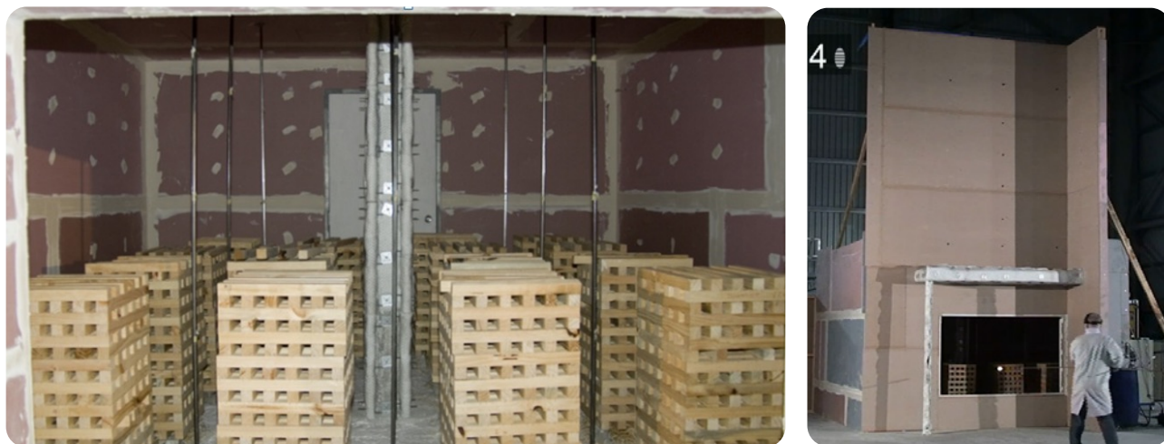
Figure 24: Typical configuration of a natural fire experiment – FWPA project PNA217-1011 73, 74 .
