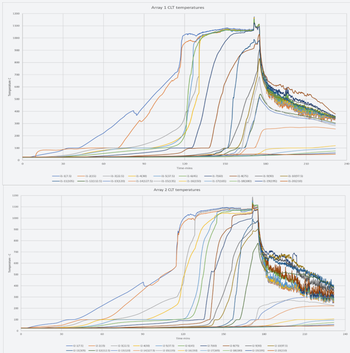
Figure 83: Thermocouple array temperatures in body of the CLT panels.
