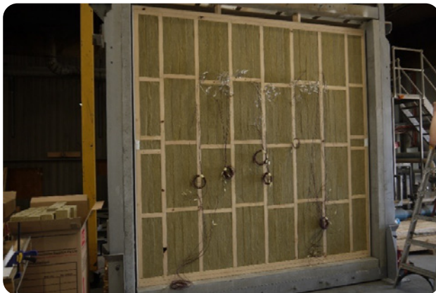
Figure 115: Internal structure and non-fire side of high-performance timber-frame wall system.
