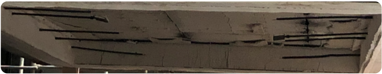
Figure 109: Most of Layer 3 of PB fallen from ceiling 2 hours after start of monitoring period.
