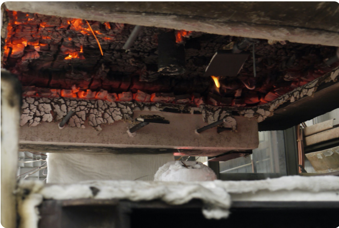
Figure 206: Fire side 18 min after completion of heating period.
