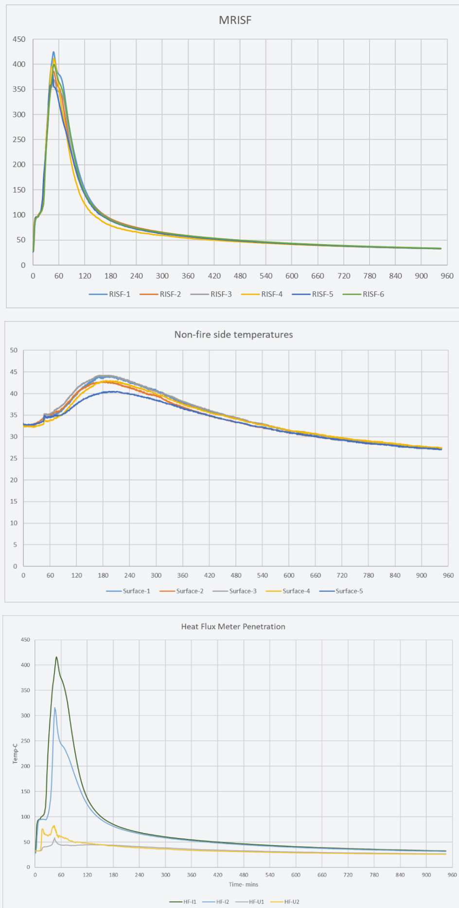
Figure 194: Modified Resistance to the Incipient Spread of Fire, non-fire side and heat flux meter service penetration thermocouple data – Test 6.
