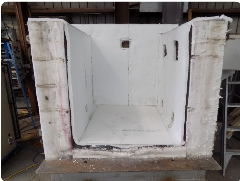
Figure 135: Test furnace with front demountable panel removed to show the interior.
