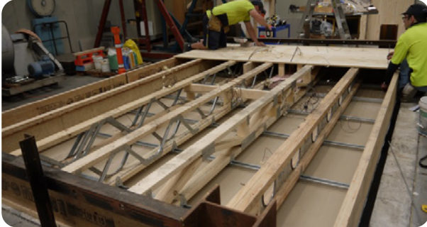
Figure 101: Timber floor test with lightweight engineered beam systems during construction and viewed from the underside before fire testing.
