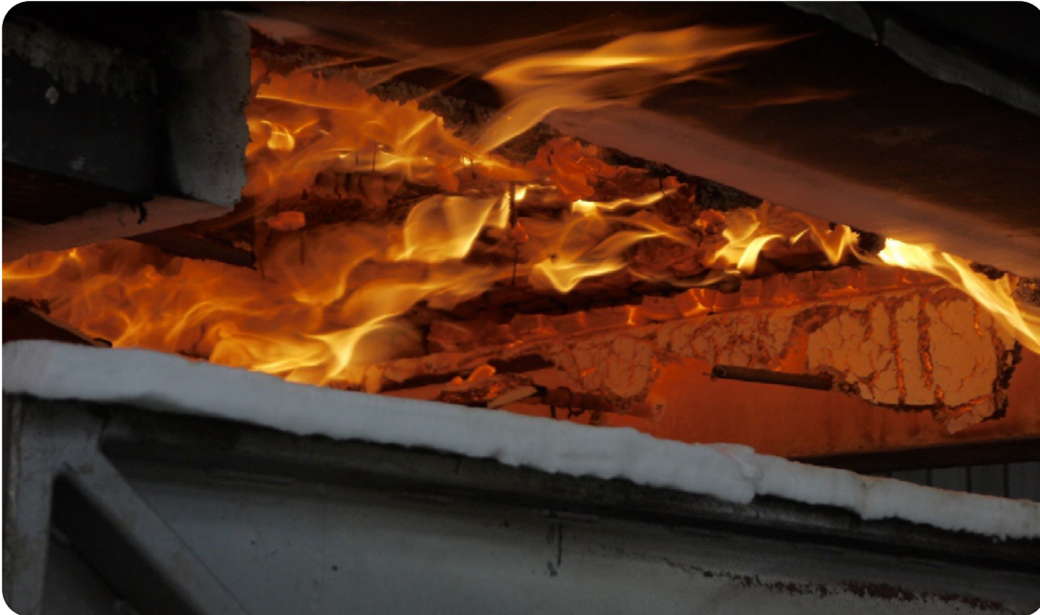
Figure 204: Fire side 6 min after completion of heating period.
