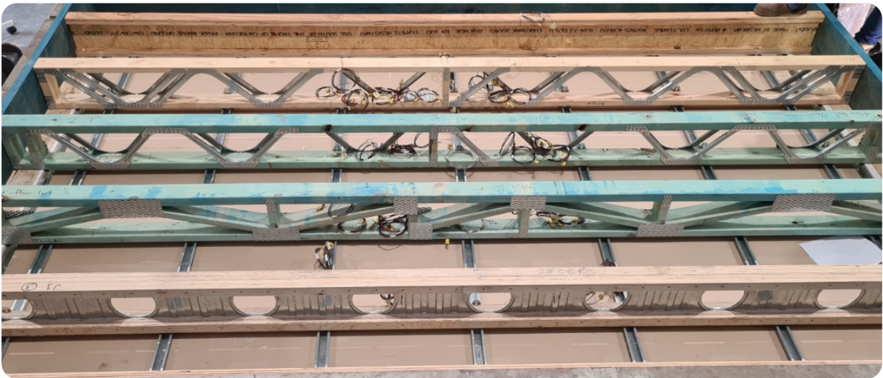
Figure 123: Test assembly before fitting flooring.
