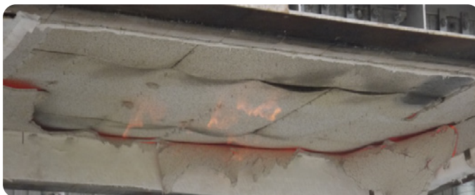
Fire-exposed face after removal from the furnace.
