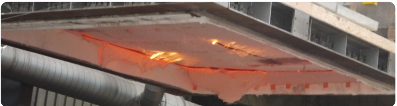
Figure 102: Specimen in process of removal from furnace 4 min after end of test (load still applied).
