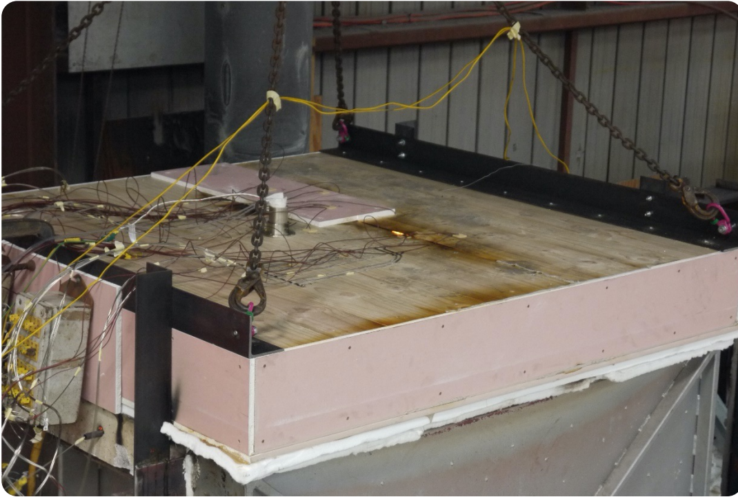
Figure 202: Non-fire side 2 min after completion of 171 min heating period.
