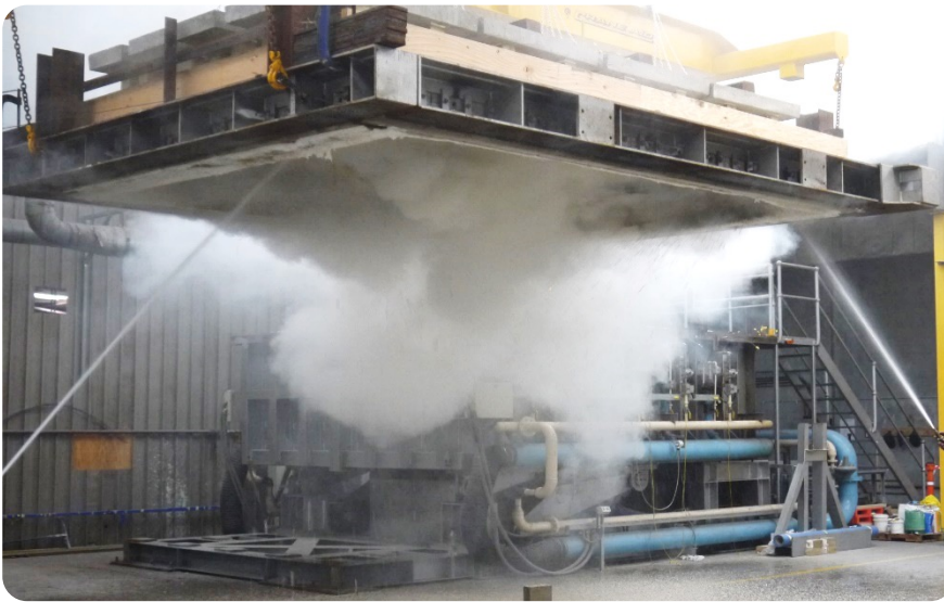
Figure 104: Application of water to specimen 6 min after test – specimen still under load.
