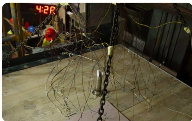
Figure 134: Non-fire side showing joint and heat flux meter service penetration.
