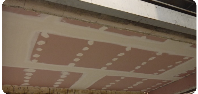
Figure 101: Timber floor test with lightweight engineered beam systems during construction and viewed from the underside before fire testing.
