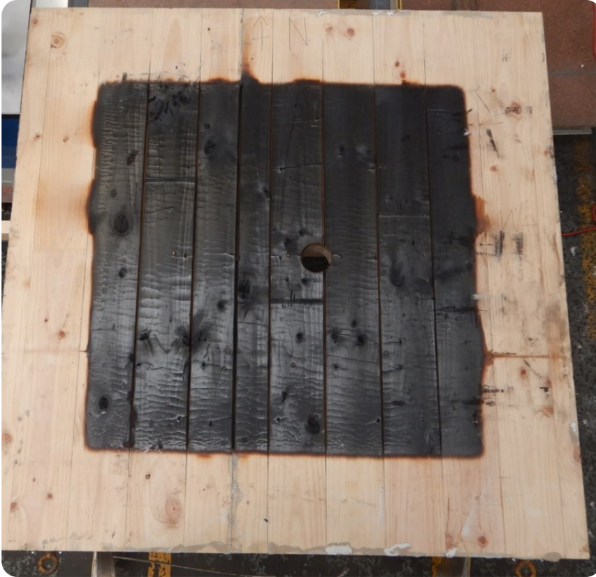
Figure 196: Fire-exposed face after completion of 15-hour monitoring period with plasterboard face removed – Test 6.
