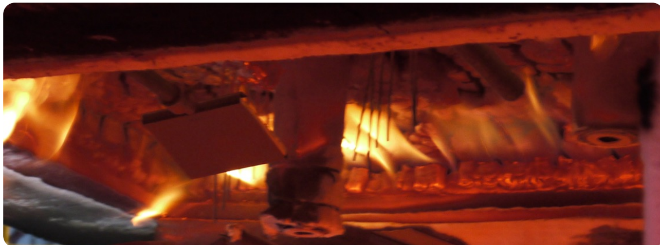
Figure 20: Underside of CLT panel after exposure to hydrocarbon heating regime, showing delamination and flaming from interface between lamellae.
