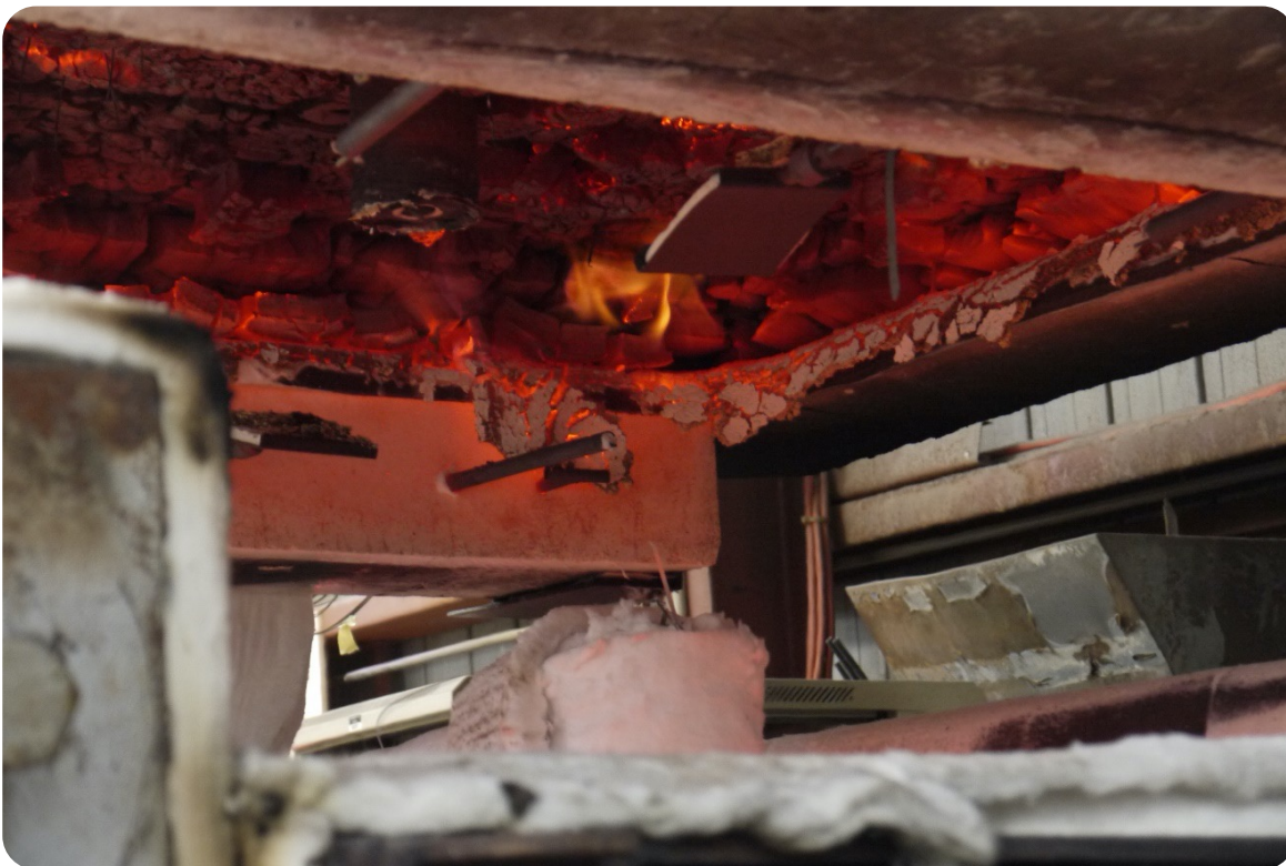
Figure 205: Fire side 10 min after completion of heating period.
