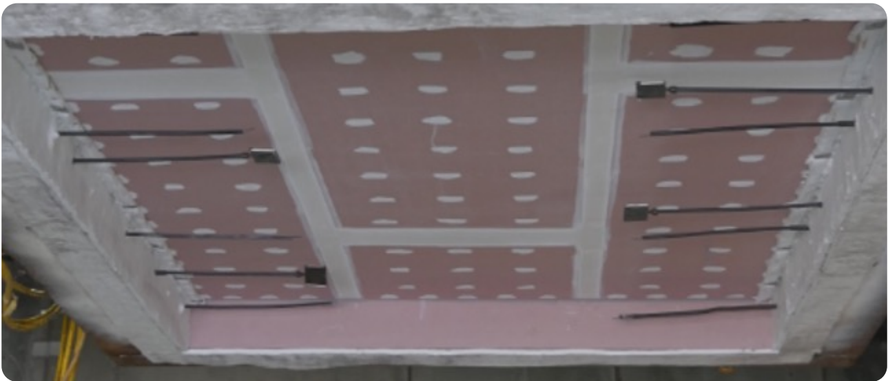
Figure 105: FRL 120/120/120 Timber floor test viewed from the underside before fire testing.
