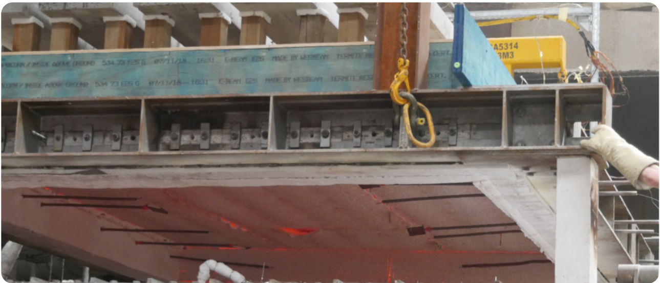
Figure 107: Specimen located 600 mm above furnace 122 min after the start of the fire test showing all layers of plasterboard in position but edges of boards sagging between fixings.
