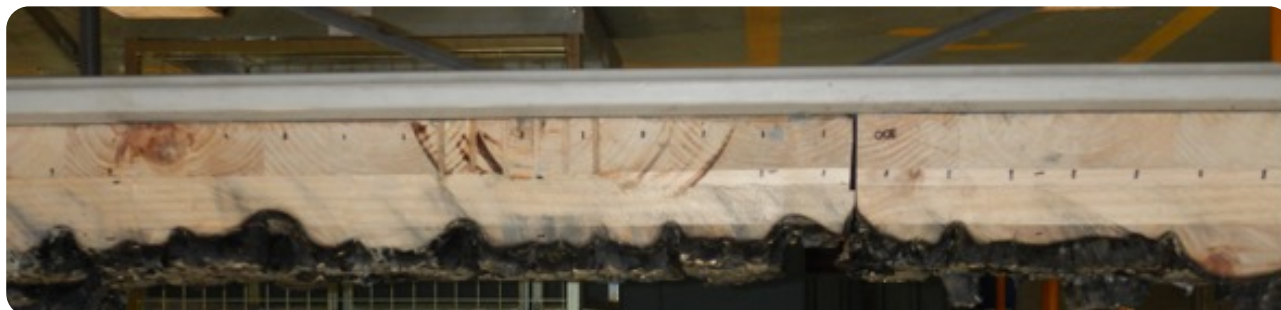
Figure 181: Cross-section of CLT at end of 120 min hydrocarbon heating regime test.
