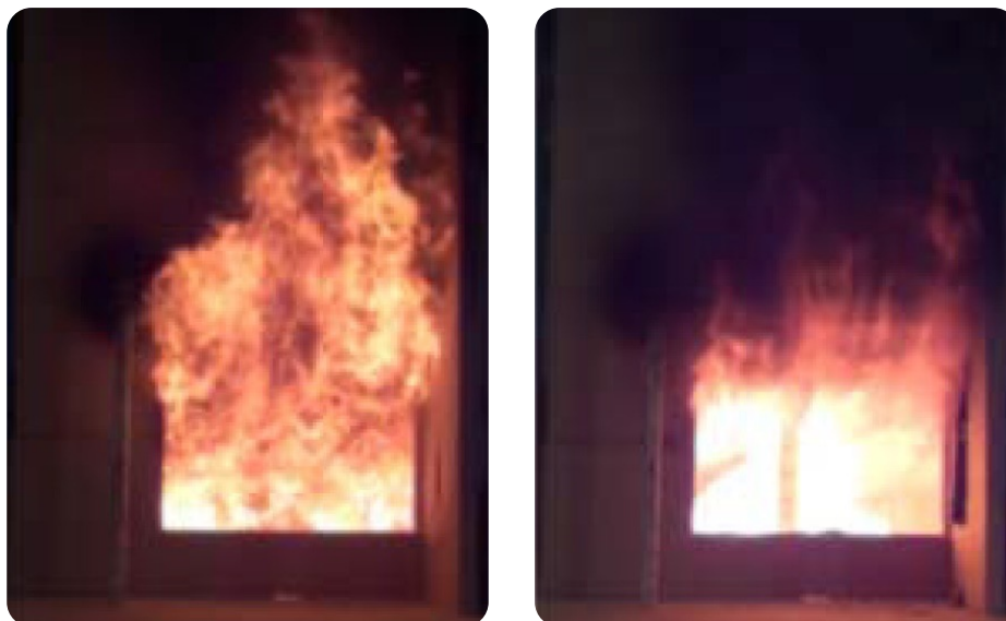
Ventilation Controlled conditions
