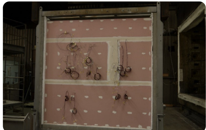
Figure 115: Internal structure and non-fire side of high-performance timber-frame wall system.
