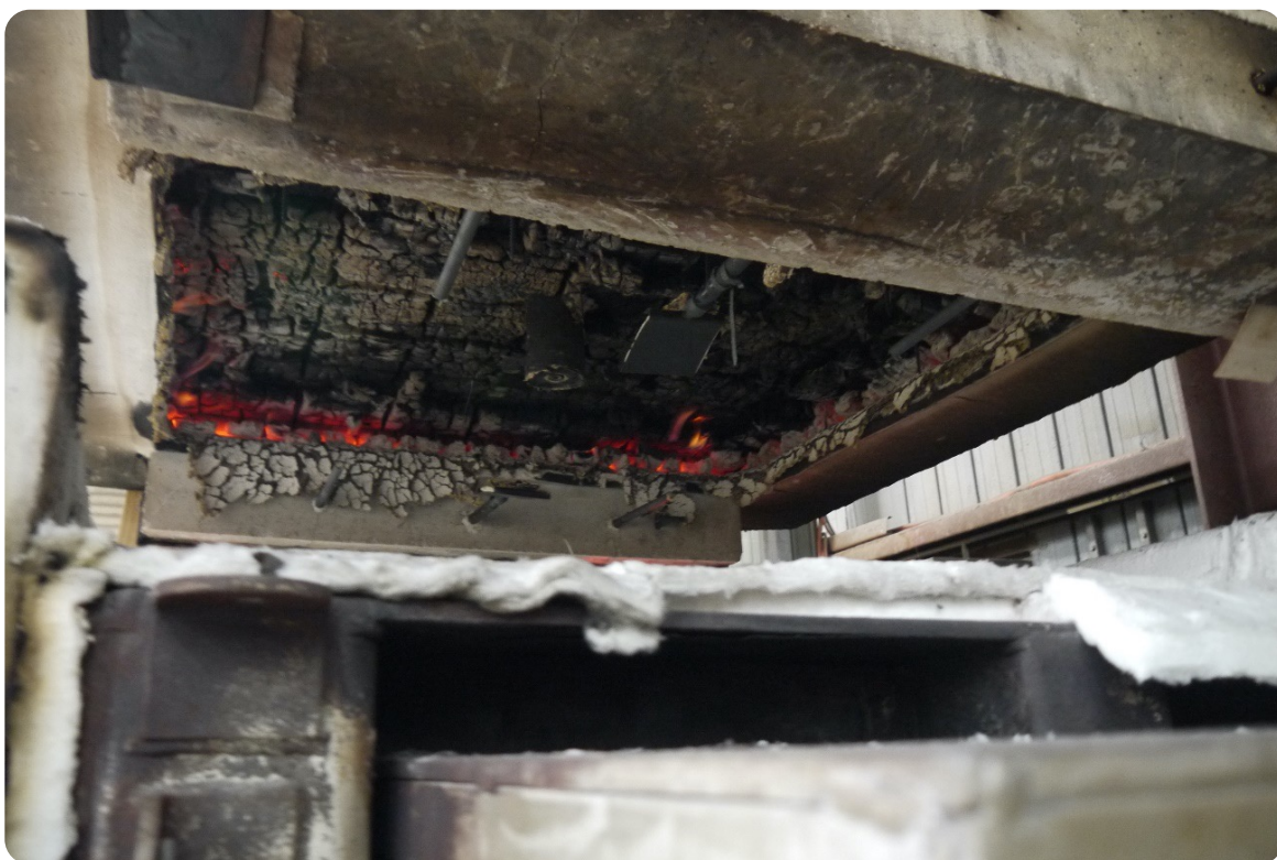
Figure 207: Fire side after monitoring period (approximately 6 min after completion of heating period).
