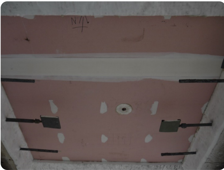
Figure 136: Typical underside of specimen before test showing furnace thermocouples and heat flux meter.
