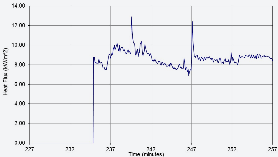
Figure 121: Heat flux measured 500 mm from the face of the specimen that was exposed to heating.
