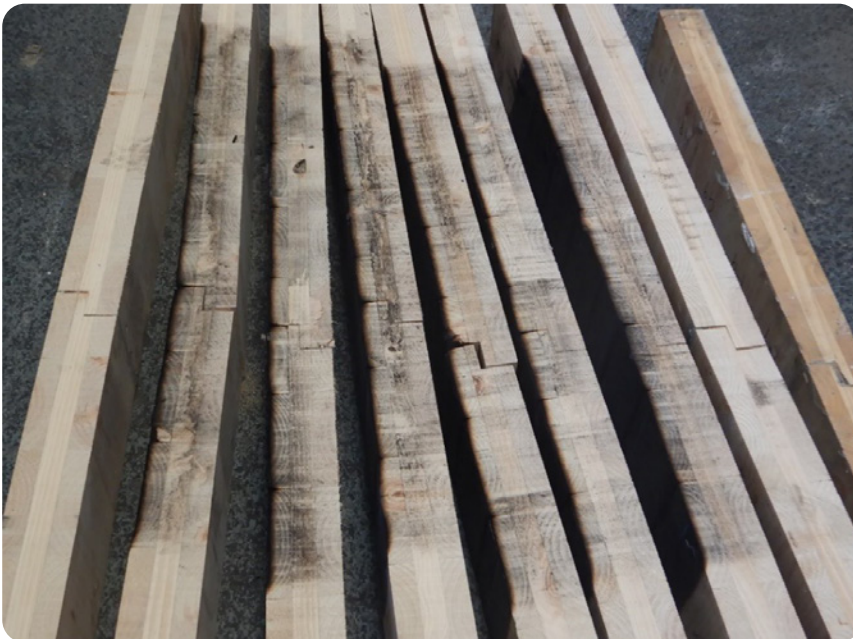
Figure 197: Sections through 105 mm CLT panel after test – Test 6.
