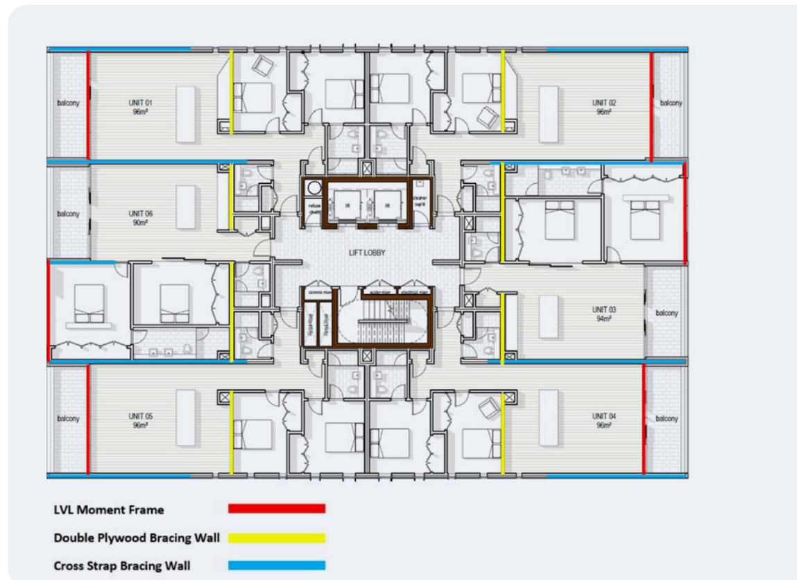
Figure 20: Level 1 Shear Wall Layout
