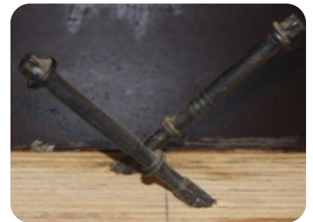
Figure 5.2: SFS screws installed at an angle of \pm 30^\circ (left) and \pm 45^\circ (right).
