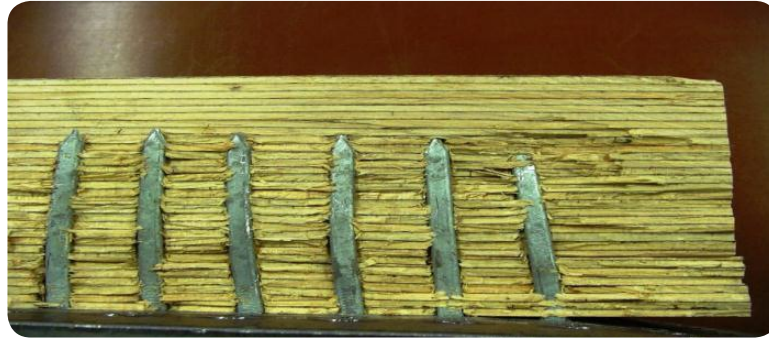
Figure 3.2: One-sided timber rivet connection.
