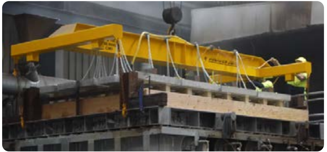
Figure E2: Lightweight loaded timber floor system after 90-minute fire-resistance test.
