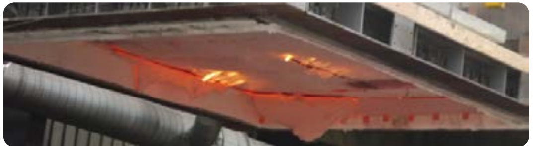
Figure E3: Fire-exposed face of lightweight loaded timber floor system after 90-minute fire resistance test.
