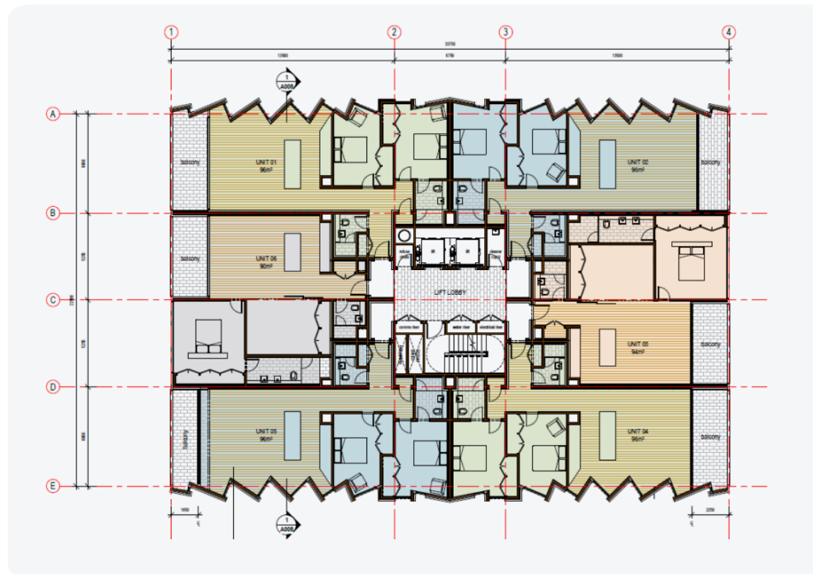
Figure 4.3: Typical CLT apartment layout
