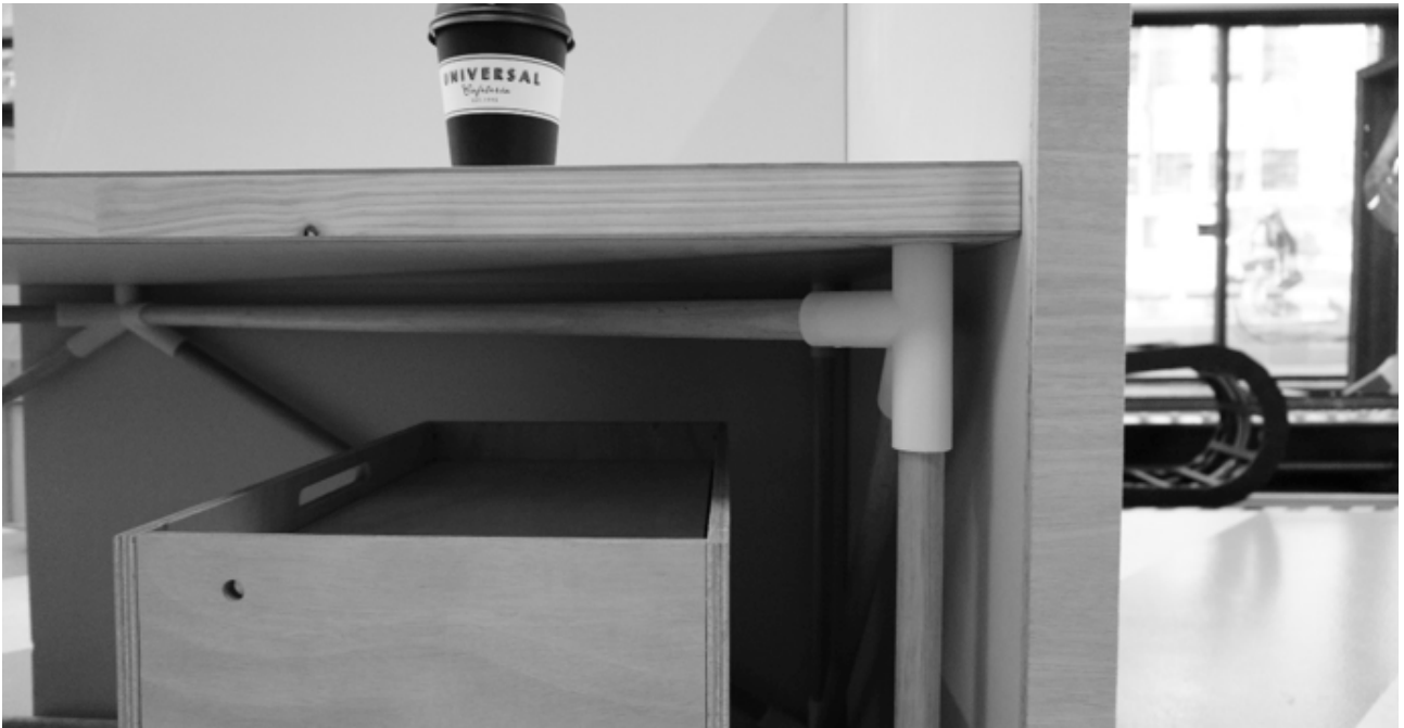
Figure 14: 3D printable joiners and dowels, UTS June 2016.
