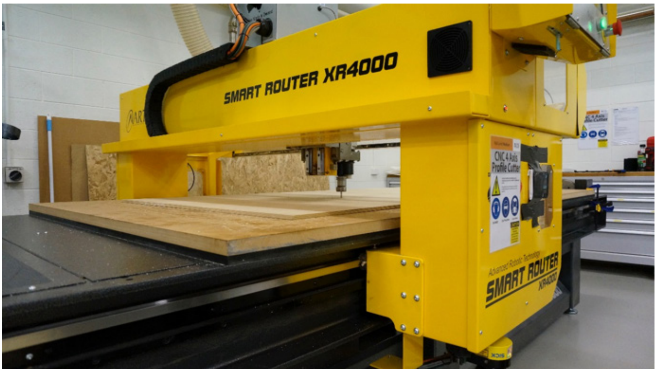
Figure 25: Open Desk Pedestal manufacture, UTS CNC milling machine, UTS 2016.
