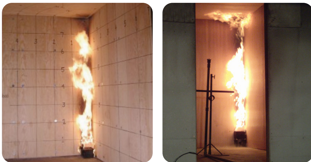
Figure 3: AS ISO 9705 fire tests.
