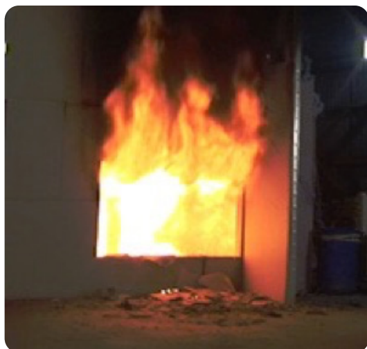
Figure 6: ISO 13785.2 test configuration.
