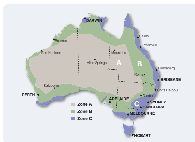
Figure 33: Hazard zone for embedded corrosion
