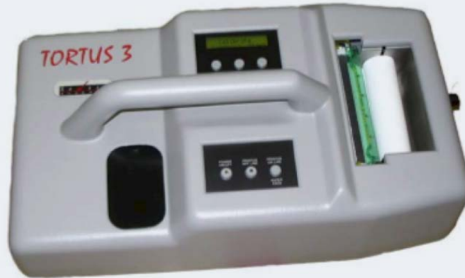
Figure 7.2: Tortus Dry Floor Friction Tester. From http://www.mastrad.com/tortus3.pdf
