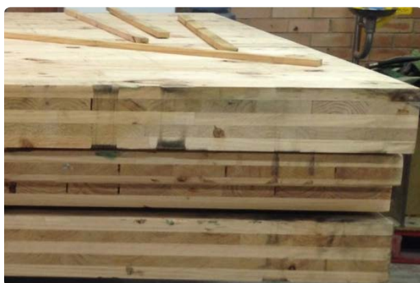
Figure 13: CLT panel arrangement: stacked panels of 5-layered CLT (left). A schematic of a 3-layered panel (right).
