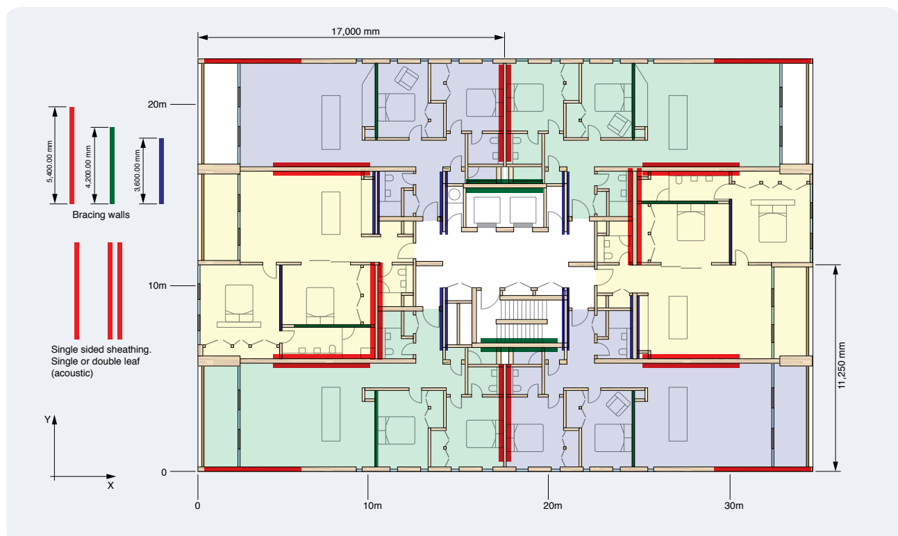
Figure 7.26: Example shear wall arrangement.
