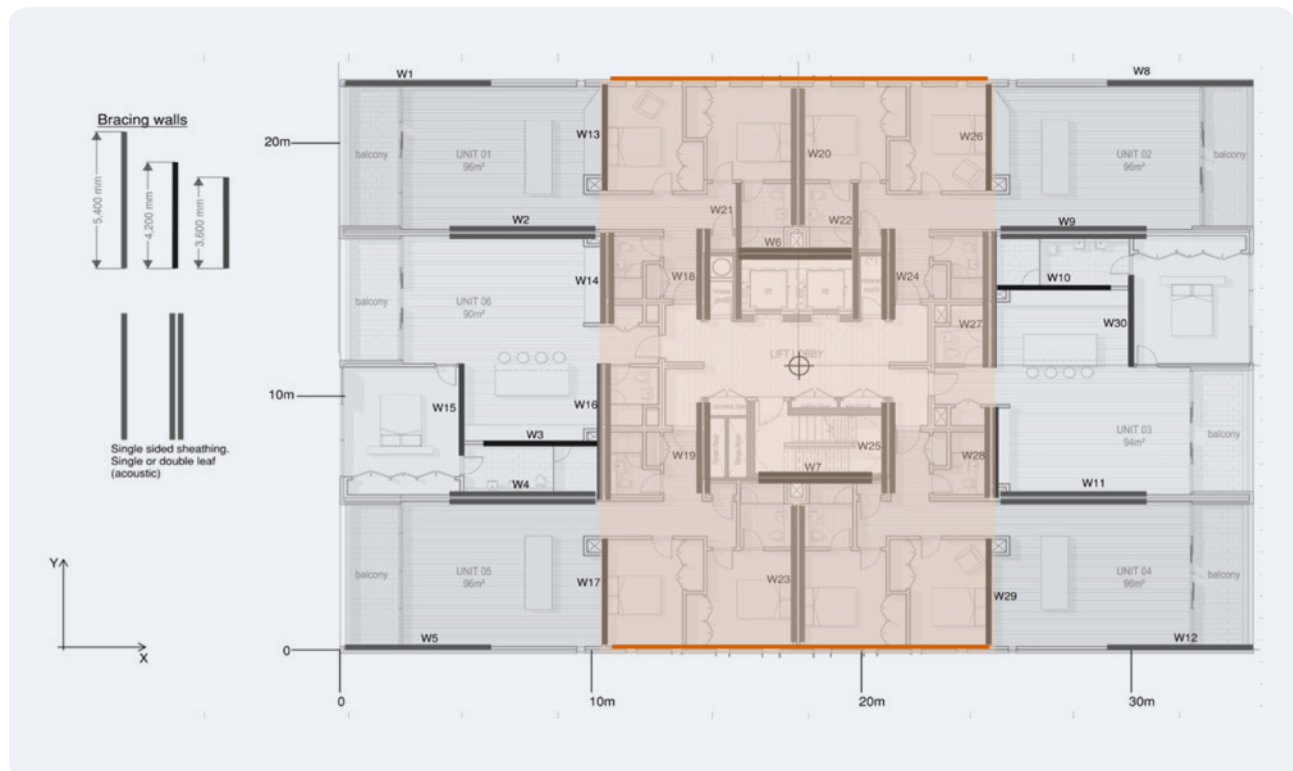
Figure 7.27: Activated bracing zone.
