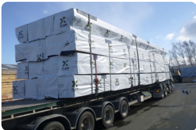
Figure 17: Mass timber elements wrapped for transport. (Image: Xlam Australia)
