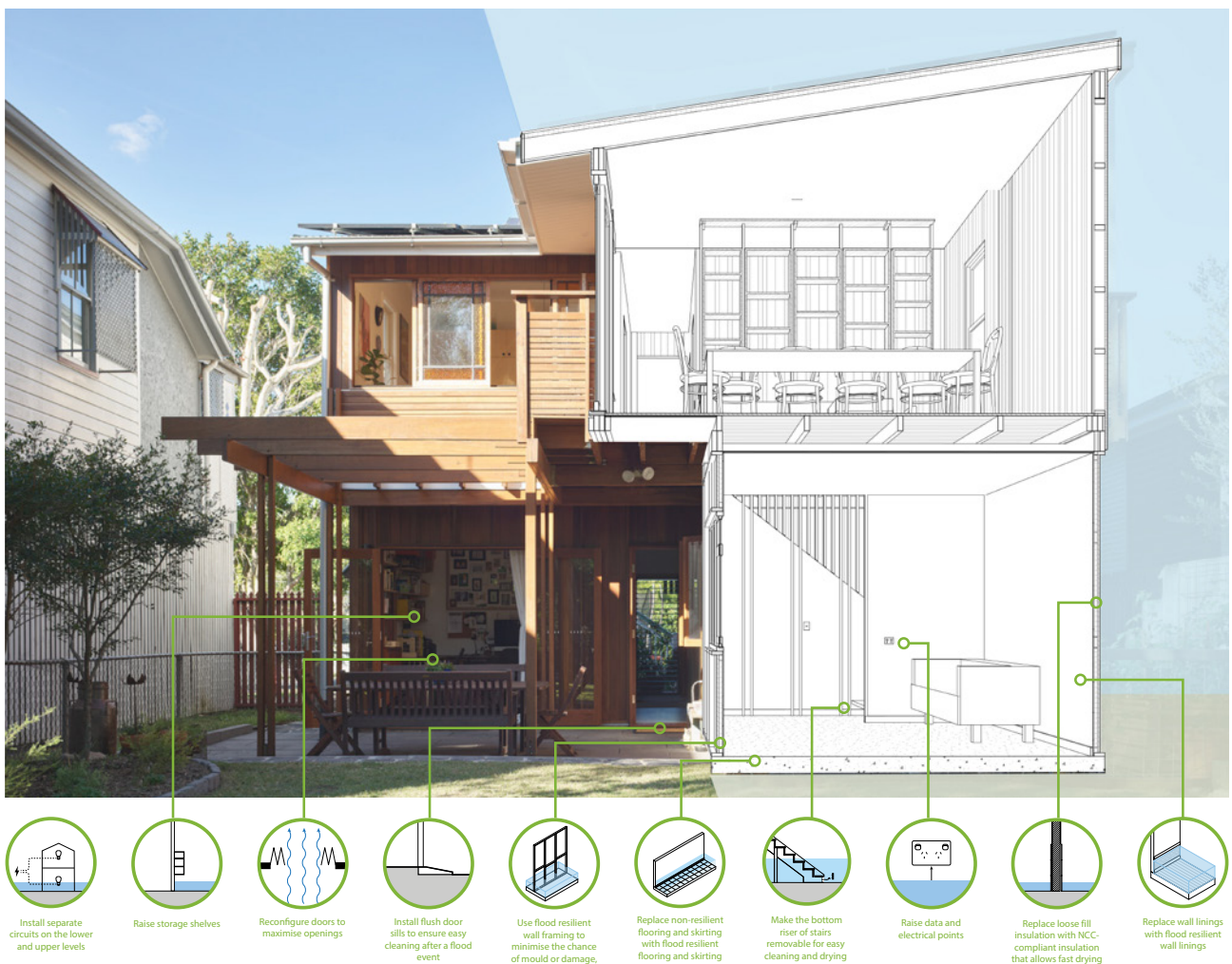
Figure A3: Summary of the flood-resilient renovation strategy at the 'Chelmer Flood House'. (Image credit: JDA)
