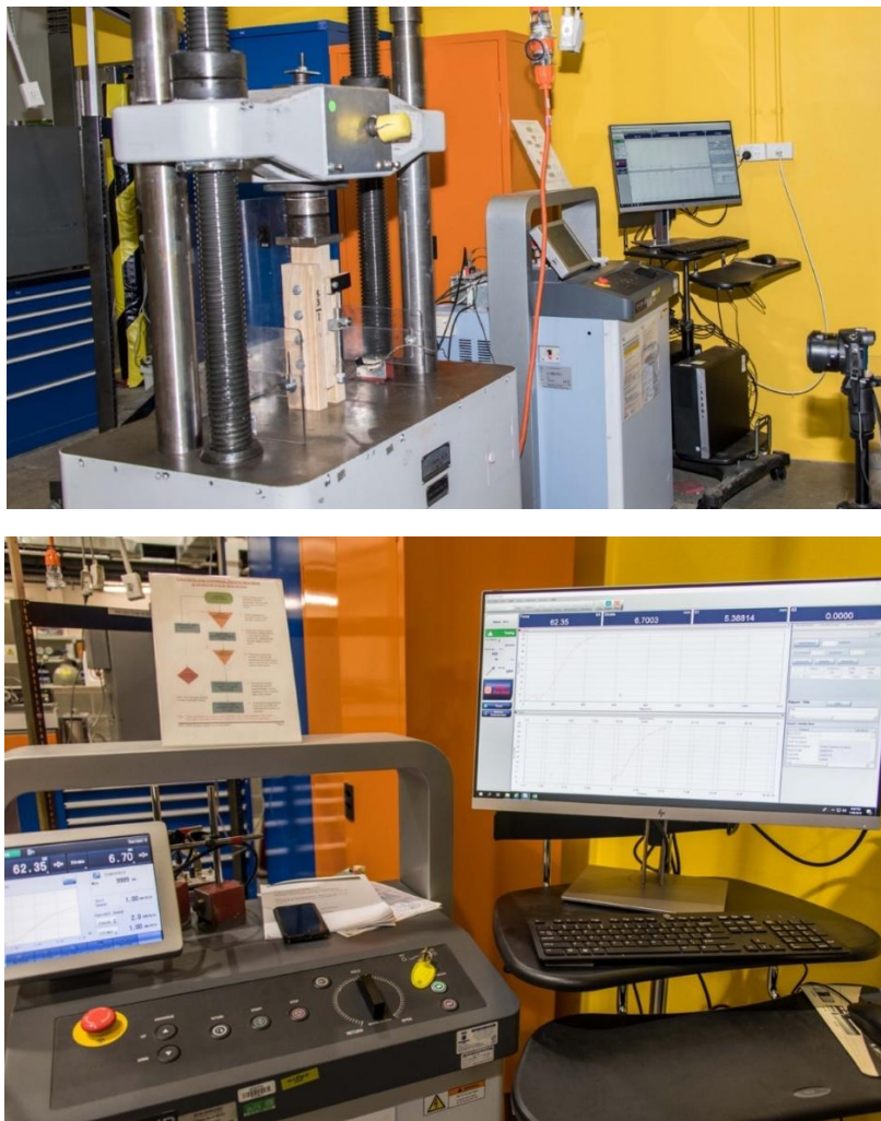
Figure F3 – Photographs of UTM and acquisition system used for compression test
