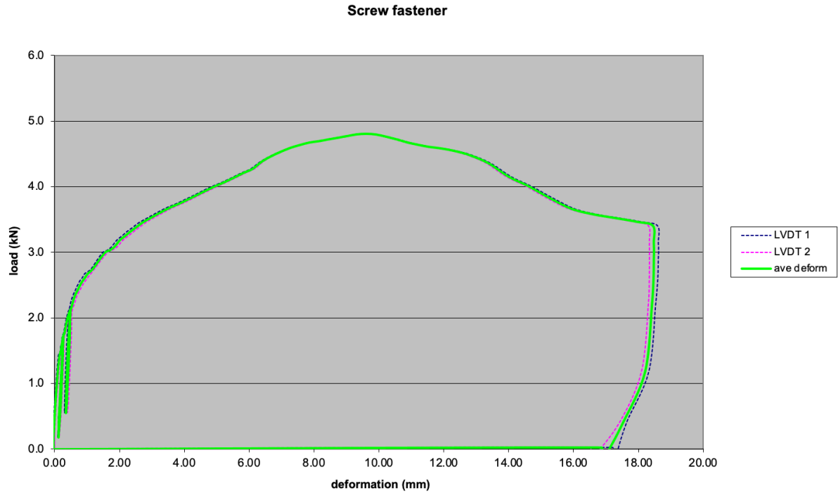
Figure E2 – Typical Load vs Deformation curves for screws
