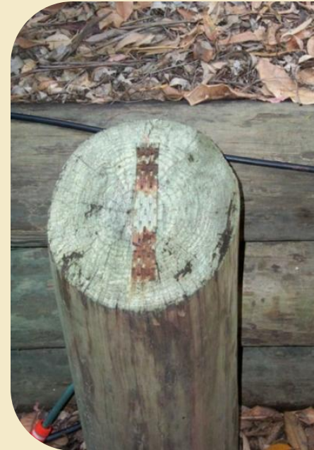
The sapwood in this pole has been treated with CCA and is causing accelerated corrosion of the galvanized plate
